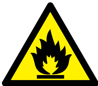
Flammable material or high temperature*
