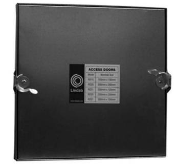
This access door fits on the flat side of a rectangular duct with fixing tabs and has a 25mm thick high density insulation. Both the door and the frame have a rubber gasket. Can achieve maximum tightness class C.
