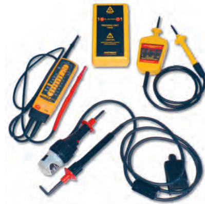
Typical devices for proving dead
