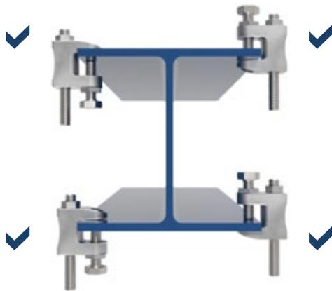
Tapered Steel Flanges – the screw has to grip on the inside of the flange.
