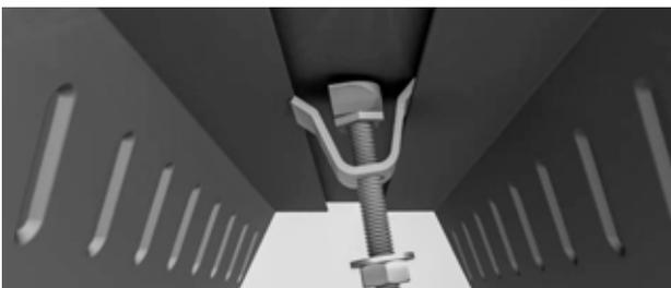
Assemble the wedge nut, locking plate and hexagon nut on the end of threaded rod and inset into the decking slot.
