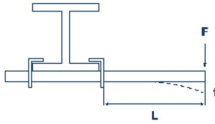
As a matter of course, loads on cantilevers should be positioned as close as practically possible to the steelwork.
