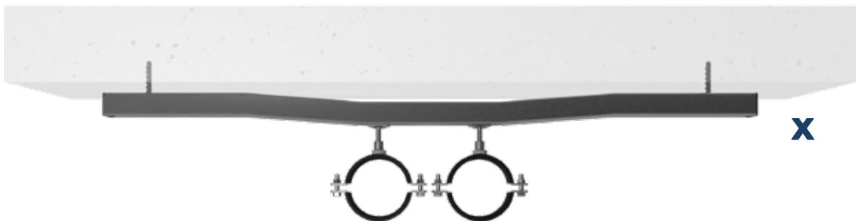
Install the anchors as close as possible to the drop rods to avoid lever arm loads acting on the header rail and anchors.
