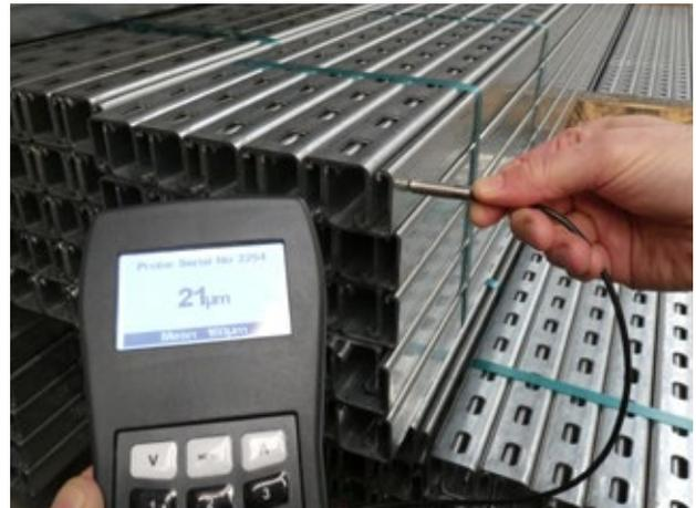
**Hot dip galvanised MX channel** is made from uncoated steel and hot dipped in molten zinc after manufacture to BS EN 1461. This gives a thicker zinc coating of at least 55 microns and means there are no uncoated edges. HDG is a tough finish and gives good corrosion protection in indoor or outdoor environments up to C4 corrosion classification.
