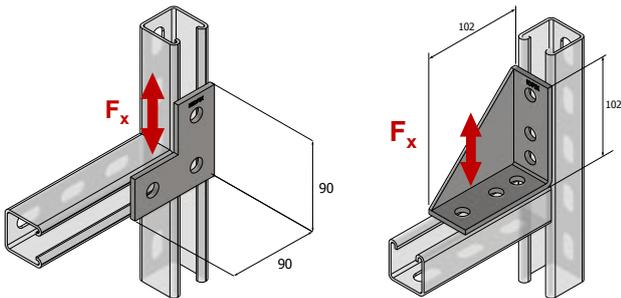
3. To realise the maximum safe working load on all MX connections the specified fasteners and required installation torque must be used.
