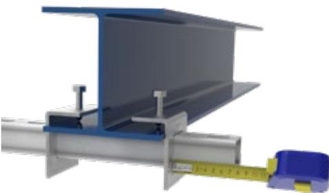
The channel must extend beyond the beam clamp by a minimum of 75mm.
