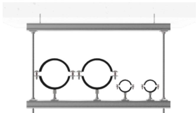
Biased load – apply total load to each threaded rod for worst-case result
