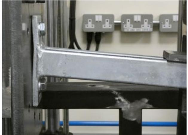
As a rule, larger pipes and service loads should always be positioned as near to the back plate as possible.
