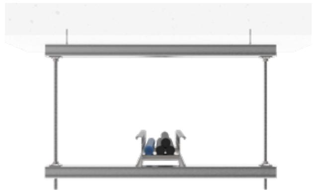
Centre Point Load – applies when the cable ladder is inside the 2-point load positions
