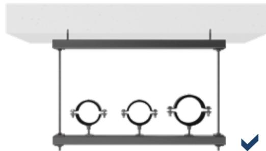
The anchors are critical components and should be specified by the relevant project engineer. The installer should make sure they have this information together with the appropriate number of anchors for each header rail.
