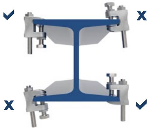
Tighten by hand + ½ turn with a spanner
