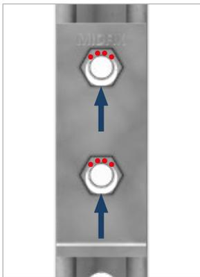
Position the set screws so that they touch the top edge of the bracket holes. This is to prevent movement of the bracket within the hole.
