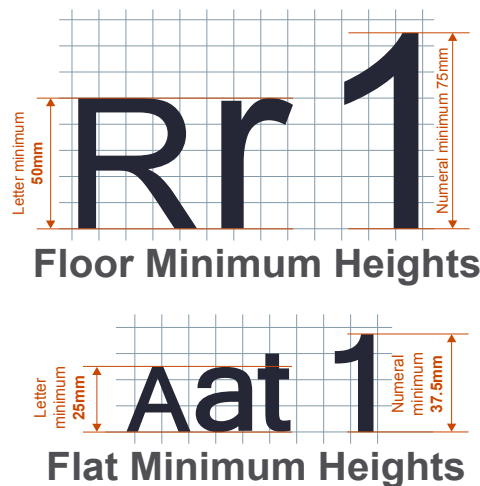
Diagram E: Example letter heights for floor and flat identification signage
