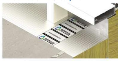
If movement is expected, an appropriate system that can accommodate movement should be used.
