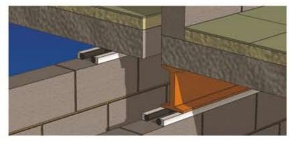
If services penetrate the head of the wall joint they need to be sealed with an appropriate fire-stopping material or product.
