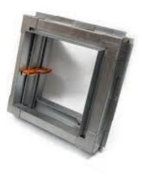
Folding curtain fire dampers are constructed so that the interlocking blades fold to the top for maximum free area in the airway, to then be released once the temperature rises (normally rated at 72C +- 4C) to fill the airway and prevent the passage of fire.
