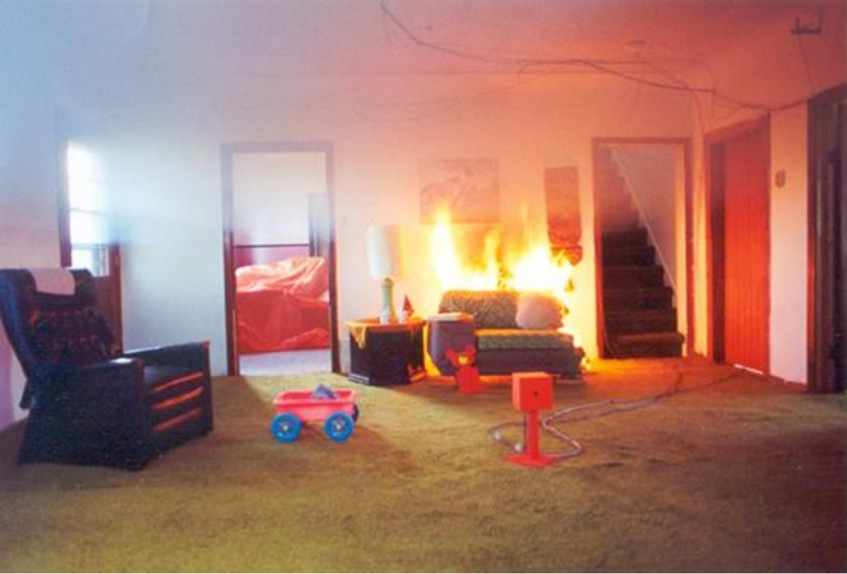
Figure 7: Fire growth in a residential test burn
