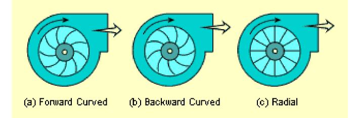
Forward curved / inclined blades (a) are curved / angled in the direction of the wheel rotation. They are most used in clean-air systems as they are particularly sensitive to particulates found in the air. They are the least noisy centrifugal fan.
